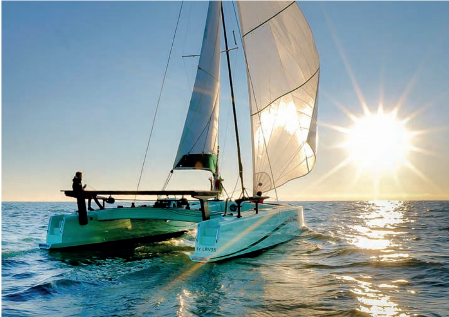
Sustainable materials can also encourage sustainable products. The LBV35 is made from Basaltex (right), a fibre extruded from volcanic rock, and is powered by sails and two solar-refuelled electric motors. Designed to fit in a shipping container, the charter catamaran can follow the sailing seasons around the world
