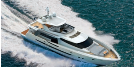
The Couach Fly 86/2600 is the largest structure built to date using Sicomin's InfuGreen 810 bio-based resin
