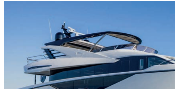
The hardtop on Sunseeker's new Ocean 90 has been made considerably lighter by using Hexcel's HexPly XF combined with HexPly SuperFit semi preg
